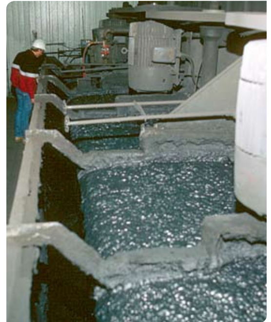
Flotation cells are used in the milling process. (Photo: Yukon government)
